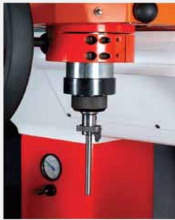
Quick holding & changing of tool holder with live pilots.
