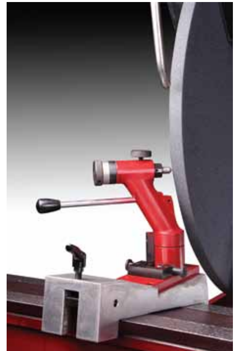
Accurate radius dressing mechanism
